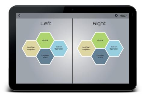
In Split Mode, you can run two magnetic field applications completely independently of each other. In this setting, the screen of the control unit is divided into a left and a right area.
