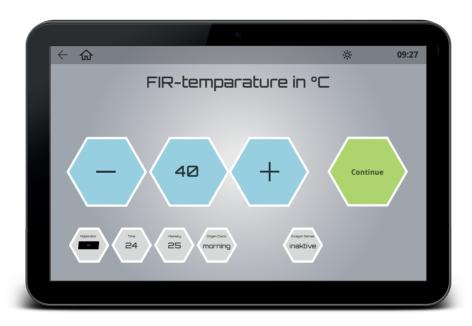
If you have a whole body infrared mat (Exagon FIR), you can use the hybrid option to start a magnetic field application with integrated infrared application. The setting parameters are expanded by the option to define the temperature of the infrared whole body mat.
